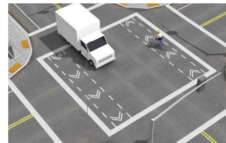
Figure 4: Possible Bike Facility Configuration Intersection Crossing Treatment (Source: NACTO Urban Bikeway Design Guide)
