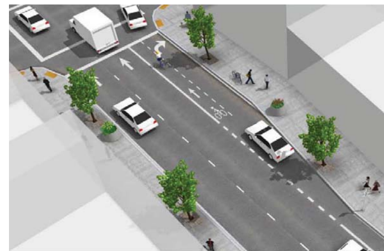
Figure 8: Combined Bike Lane/Turn Lane at Intersection (from NACTO Urban Bikeway Design Guide)
